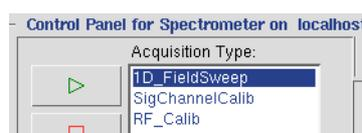
Figure 10-8 Selecting the 1D\_FieldSweep experiment.
