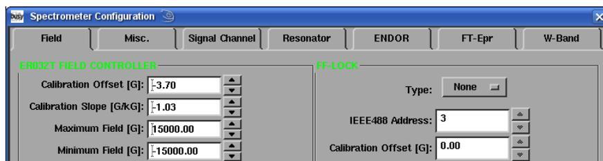
Figure 10-21 The field calibration parameters under Spectrometer Configuration>Field>ER032T Field Controller.
