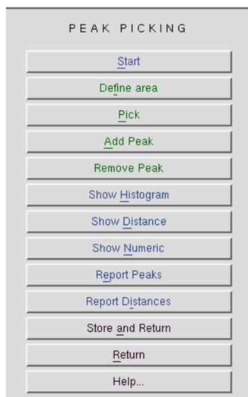
Figure 7-8 The available operations for peak picking.
