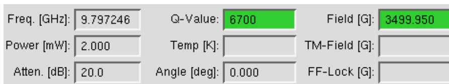
Figure 3-14 The microwave bridge status section with the Q-value display.
