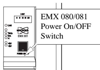
Figure 3-33 The power switch for EMX 080/081 magnet power supplies.
