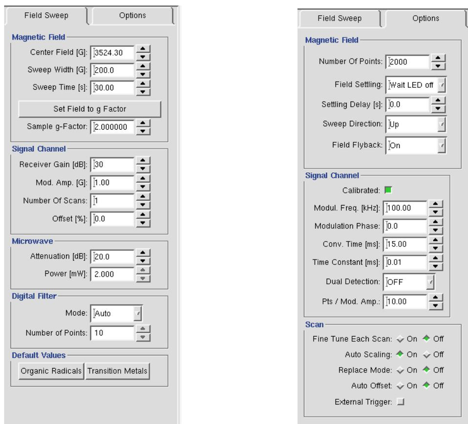
Figure 2-33 Default spectrometer parameters for organic radical samples.
